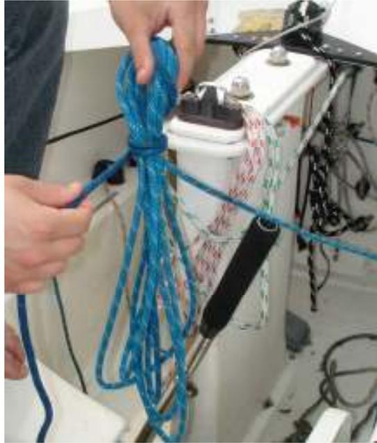
3) In order for the rope to keep itself coiled, you need to secure it at the end by doing a simple knot.
