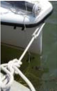
Painter or Bow line which is a line that is attached to the bow of the boat and is used to tie a
