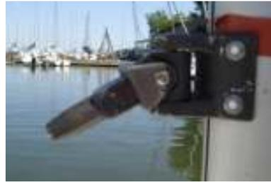
Automatic bailer: this type of bailer is usually found on the bottom of the cockpit on small dinghies.
