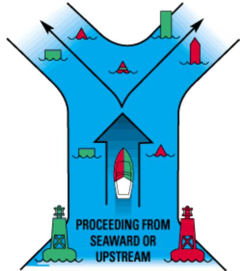
Other important buoys that you should know about are bifurcation buoys. These buoys have green and red bands on them. When passing one of these buoys, it is the top band that will define which channel is safer. For example, if a green band is on top, the safest way is to pass on the starboard (right) side, and keep the buoys on your port side (left side).
